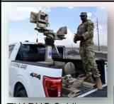
TXARNG Soldiers are enhancing their capabilities along the Texas border with the deployment of the Modular Mobile Surveillance System. (M2S2). The M2S2 is an all-terrain truck with which operates under the cover of night, thanks to its low-light, highdefinition camera, infrared camera and radar.
